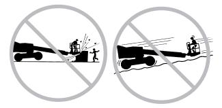
Limit travel speed according to condition of ground surface, congestion, slope, location of personnel, and any other factors which may cause collision.
