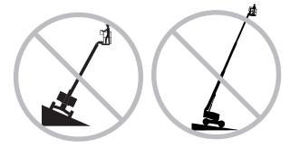
The tilt alarm sounds in the platform only when the machine is on a severe slope.
