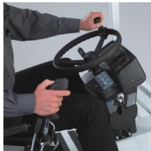
Effective control of the machine: steering with one hand while controlling the tools with the other
