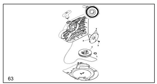
Remove the valve housing (see chapter "Replacing the starter rope").
