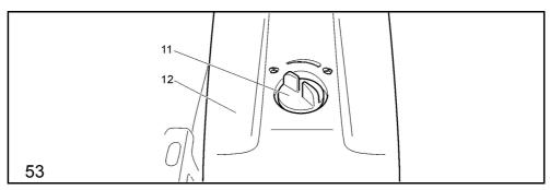
Turn the cover lock (11) to the "unlocked <sup>®</sup> " position and carefully remove the filter cover (12).
