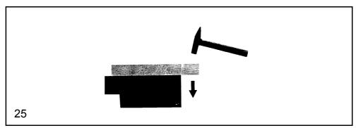
4.11.3 When truing stone slabs you only need to grind one groove (to prevent unnecessary dust formation), and then place the slab on a flat base and knock off the overhanging piece (25).
