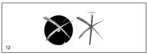
4.6.6 The cutting blade must be completely undamaged (12). Test it by performing a sound test with a piece of wood.
