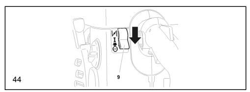
Press the multifunction switch (9) down to the "Stop" position.
