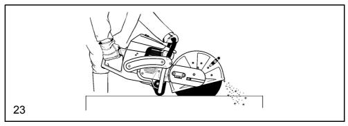
The quick rotation of the cutting blade at the contact point tears the material and throws it out of the cutting groove. As far from the cut as possible (behind it), swivel the protective hood down (23) to divert the workpiece particles that have been cut away from the operator.
