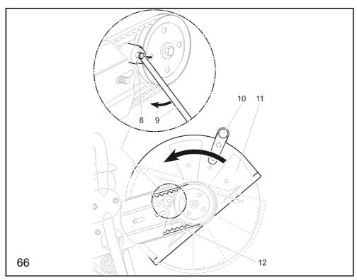
Pry out the stop pin (8) with the combination wrench (9) far enough, as shown in the figure, so that you are able to turn the protective hood (11).
