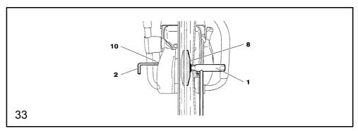
Set the clamping disc (8) onto the shaft, screw in together with the screw (32/9) and tighten by hand.
