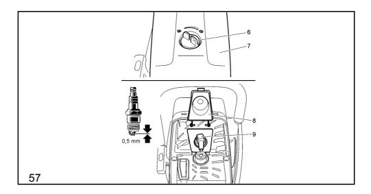
Turn the cover lock (6) to the "unlocked <sup>©</sup> " position and carefully remove the filter cover (7).
