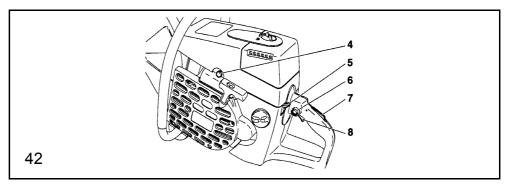
Press the multifunction switch (5) upward (choke position).
