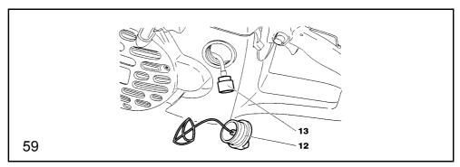
The felt filter (13) of the suction head can become clogged during operation. To ensure an unrestricted flow of fuel to the carburetor, the suction head should be replaced about every 3 months.
