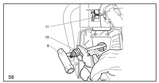
Insert the combination wrench (9) between the hood and cylinder, as shown in the figure.
