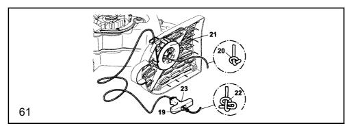
Feed in new rope with a diameter of 4.0 mm (0.16") and a length of 1,000 mm (40"), as in the illustration (do not forget the disc (19)) and knot both ends.
