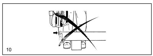
4.6.2 Cutting blades are only designed to cut materials on their edges. Never use the side surfaces for grinding purposes as this can break the disc! (10).
