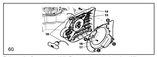
Release the four screws (14). Remove the valve housing (15).
