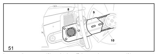
Loosen the screws (8) and take off the crankcase cover (9).
