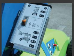
MULTIFUNCTION CONTROL PANEL IN OPERATOR-FRIENDLY DESIGN WITH INTEGRATED BUTTONS AND SIGNAL LIGHTS, DOUBLE ACTION SAFETY KEYS AND GYRO FUNTIONALITY ARE BOTH IN THE STANDARD SETUP ON THE WINLET 575.
