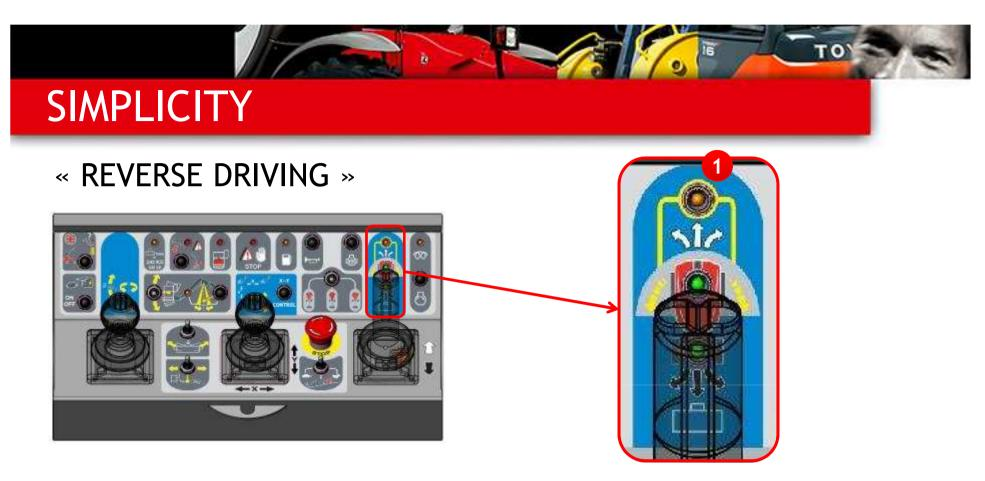
$\checkmark$  When the turret is more than 90° with the chassi, LED 1 light up Red
