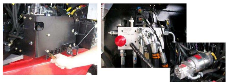
✓ Use of electric pump and action on the valve bank directly
