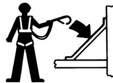
Occupants must wear a safety belt or harness and comply with applicable governmental regulations. Attach lanyard to the anchor provided in the platform.
