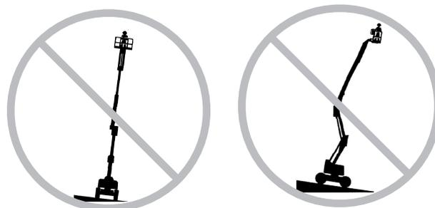
Do not depend on the tilt alarm as a level indicator. The tilt alarm sounds in the platform only when the machine is on a severe slope.
