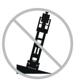
Do not use the platform controls to free a platform that is caught, snagged or otherwise prevented from normal motion by an adjacent structure. All personnel must be removed from the platform before attempting to free the platform using the ground controls.
