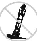
Do not use the platform controls to free a platform that is caught, snagged or otherwise prevented from normal motion by an adjacent structure. All personnel must be removed from the platform before attempting to free the platform using the ground controls.
