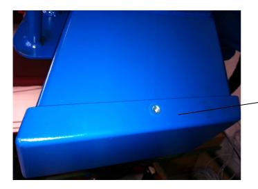
Remove cover to acces the grease nipples
