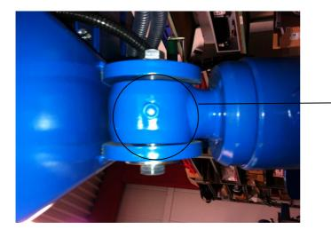
Grease main cylinder at top and bottom.
