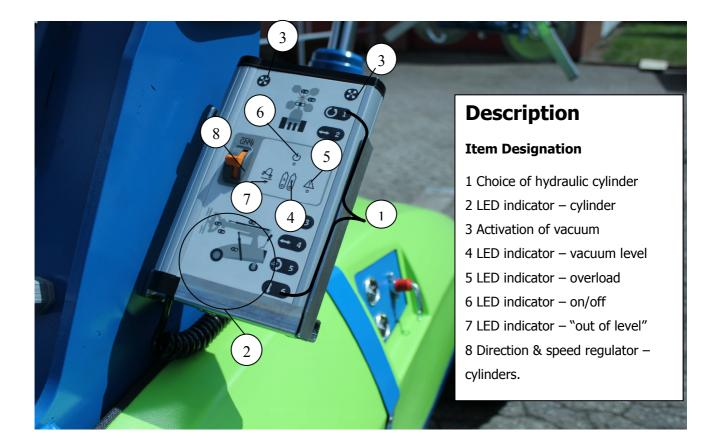
The WinLet 575 is equipped with an operating panel from which all vacuum and hydraulic functions are controlled. The integrated safety functions are:
