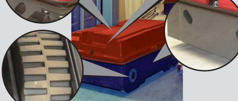
Improved chassis design, now 15mm plate with heavy duty winch and tie down points making life easier for transportation
