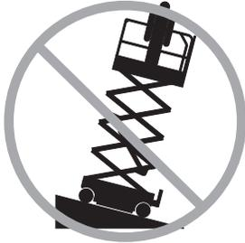
Do not raise the platform unless the machine is on a firm, level surface.
