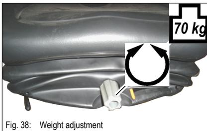
Fig. 38: Weight adjustment
