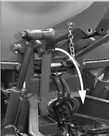
Fig. 26: High-tip skip maintenance strut
