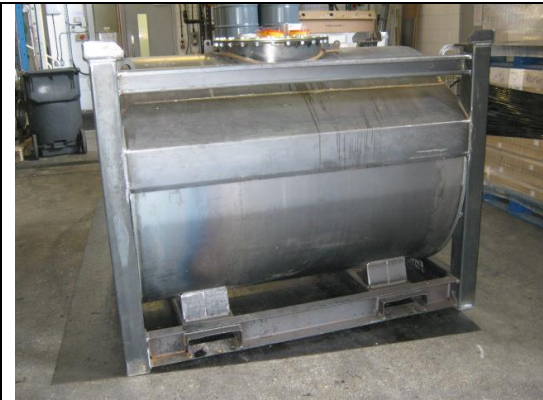
950 litre mild steel IBC submitted for performance tests
