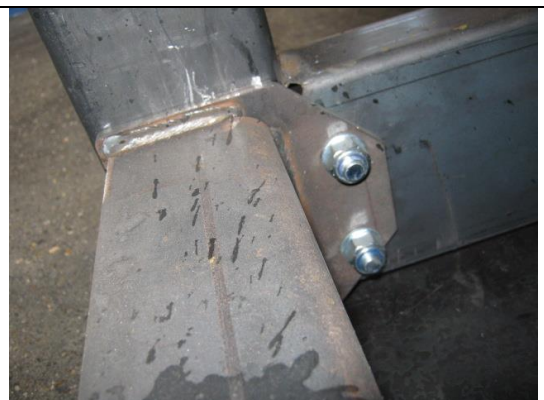
Bolted attachment for outer and inner sections
