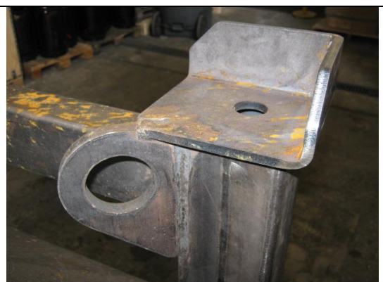
Stacking plate at top of corner post
