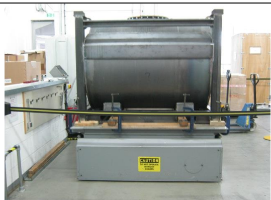
IBC vibration test
