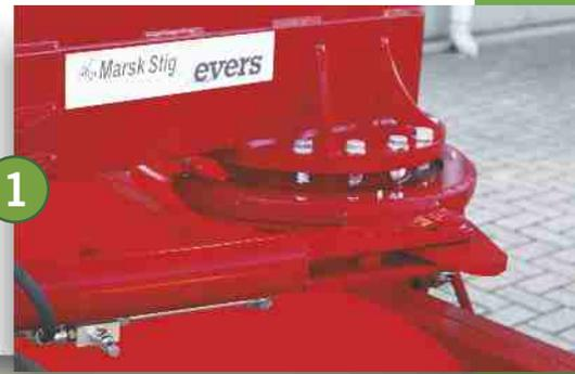
Hydraulic adjustment of the blade, easy to control.
