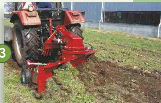
Easy to work under different conditions by simply adjusting the angle of the blade at Proff version.
