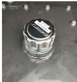
Figure 5-5 Hydraulic Tank Breather
