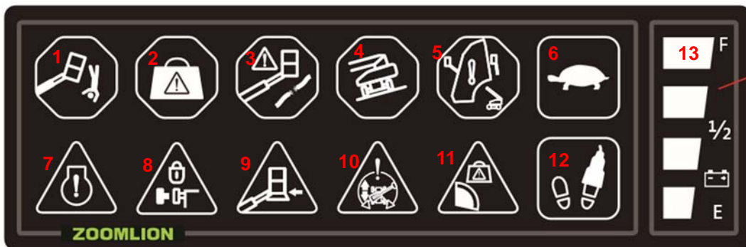
Figure 2-13 Platform Control Indicator Panel
